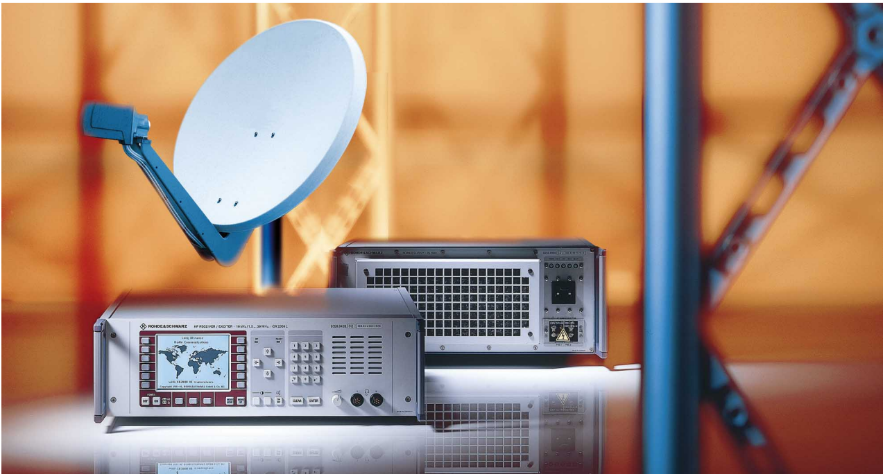
FIG 2 SpaceMan DS101 system for combined shortwave-satellite transmission consisting of HF Transceiver XK2000, PC with Message Handling Software PostMan, decoder and satellite dish
