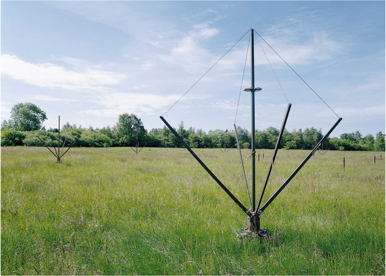
FIG 2 Combination of correlative interferometer ADD011 and Adcock antenna ADD012
