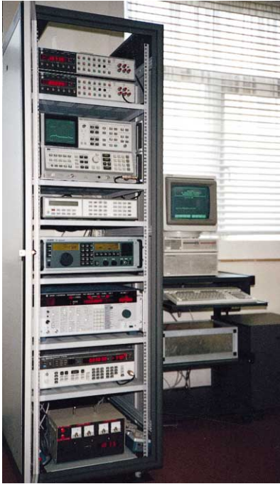
FIG 2 HF occupancy measurement system of UMIST; at the core of the system is Rohde & Schwarz Test Receiver ESH3
